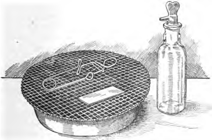
FIG. 11. STAINING DISH AND DROPPING BOTTLE FOR STAINS An enameled-ware basin covered with \frac{1}{4} -inch-mesh galvanized wire cloth
